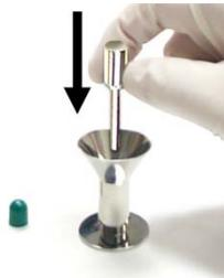
4. When the required quantity of powder has been put into the funnel, use the Tamper to compress filling material into capsule body.
