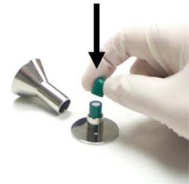
6. Place the capsule's cap onto the body of the capsule, pressing firmly to lock. Remove the filled capsule from the Holder.
