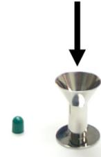
3. Dose a pre-measured amount of powder into the capsule through the Funnel, **or** put the assembly on a precision balance, tare it, and dose the powder into the capsule through the Funnel.
